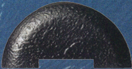
4 inch bumper w/ 0.625 x 2 inch wide groove nominal
